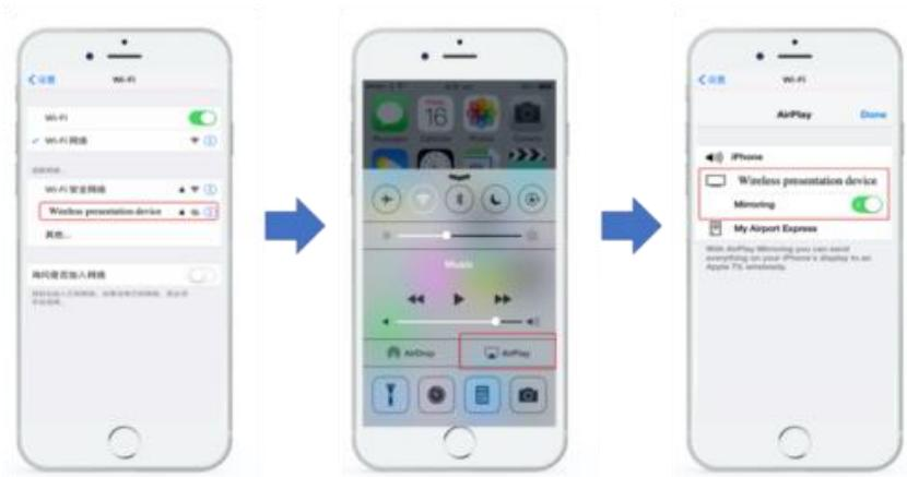
Step1: Search RX SSID and connect with the iOS devices. (SSID: RXxxxxxx, Password: 12345678), the SSID show on the left upper corner of the screen.
