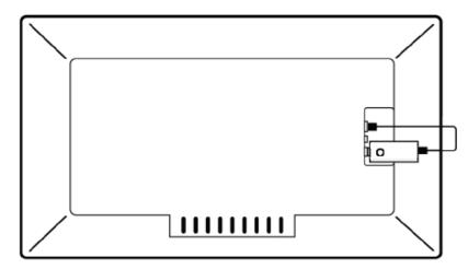
Remark: the power supply of RX is about 5V/0.5A. Please connect the RX with a power adapter if your TV can't supply enough power.
