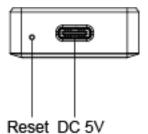
1.Reset: press the button up to 3s for factory reset
